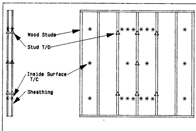
NOTE 1—The diagram shows a total of 54 thermocouples. Forty of the thermocouples provide panel surface temperatures, 14 of the thermocouples provide stud surface temperatures.
