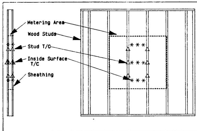
NOTE 1—The diagram shows a total of 30 thermocouples. Eighteen of the thermocouples provide panel surface temperatures, twelve or more of the thermocouples provide stud surface temperatures. As few as 3 thermocouples minimum, per side, may be used to measure stud surface temperature.
