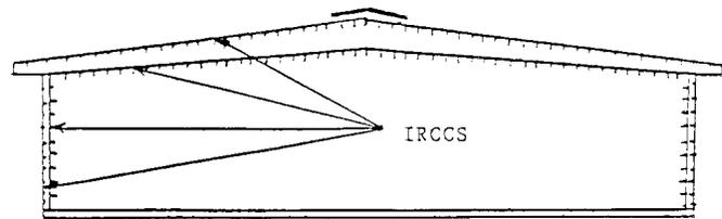
NOTE 1—Apply the IRCCS to cover the entire interior surface area. The low-emittance surface of the IRCCS must face the interior of the bldg.
