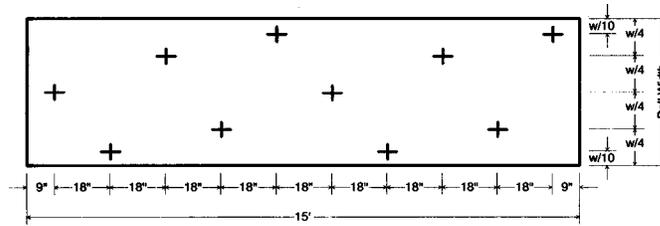
FIG. 3 Thickness Measurement Locations – Full Roll
