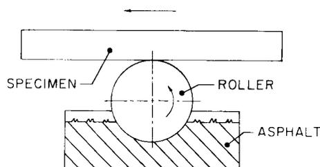
FIG. 1 Application of Hot Asphalt to Specimen Surfaces
